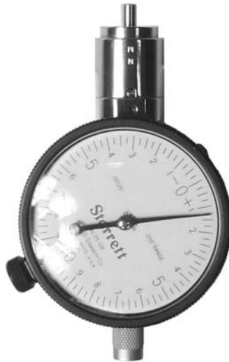
Figure G-6 Using the connector gage
